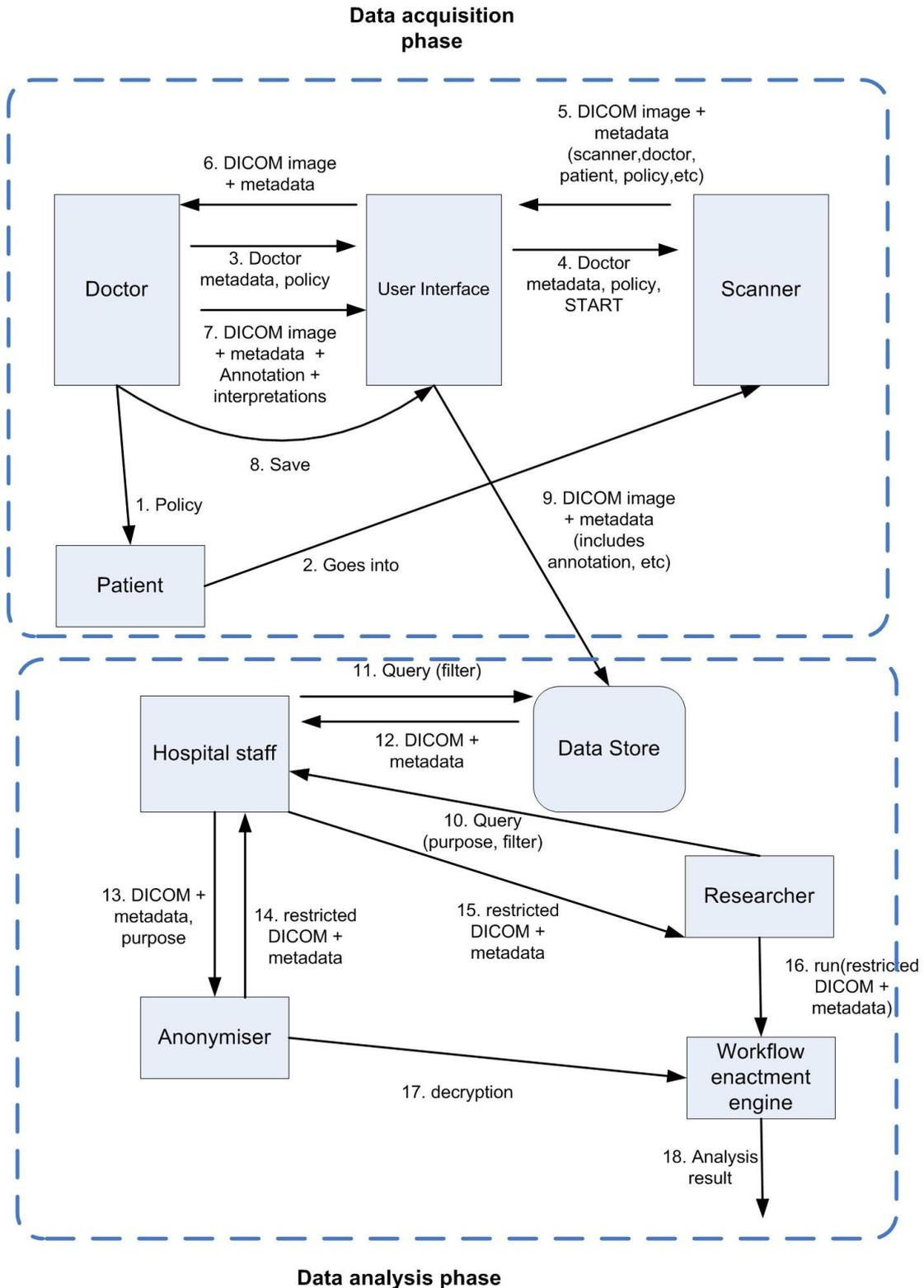
Figure 2: The actors, data and data flow making up the workflow
