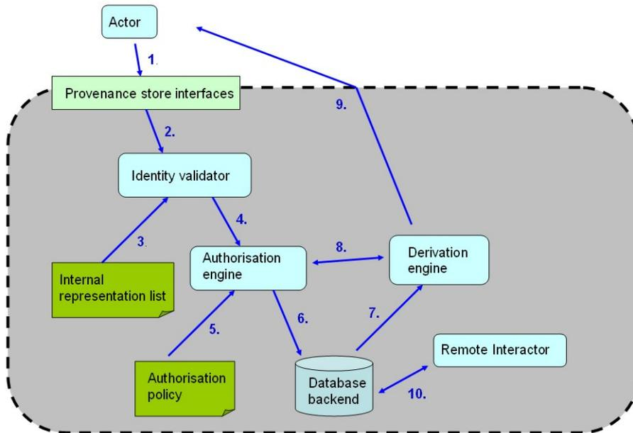
Figure 3: Security architecture for a provenance store
