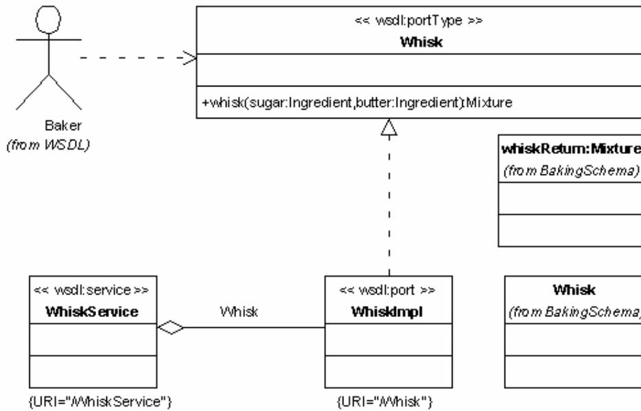
**Figure 14** The UML model of the Whisk service
