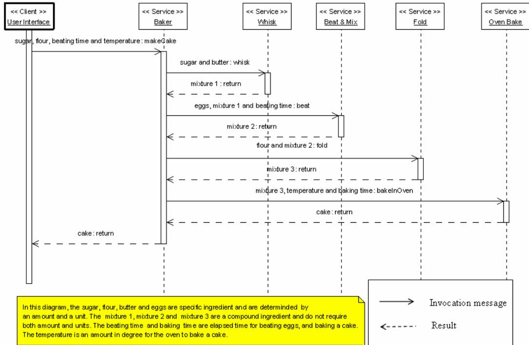
**Figure 2 The BVSC process sequence diagram**
