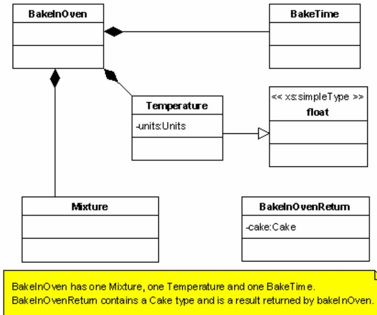
Figure 11 The UML model of the BakeInOven message
